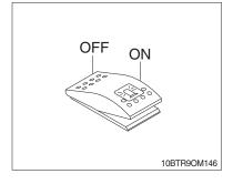
(1) This switch turns ON the rotary light on the cab.
