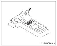
(1) When pressing the emergency switch downward the electric circuit is broken, all electrical function switch is off.
